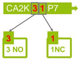
is a TeSys K auxiliary contactor, with **3 NO** contact and **1 NC** contact, 230 V AC coil
