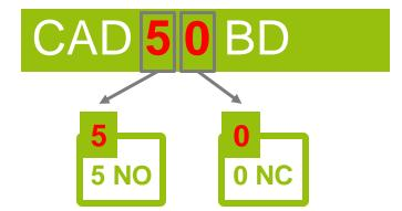
TeSys D auxiliary contactor with 5 NO and 0 NC contacts, 24 V DC coil
