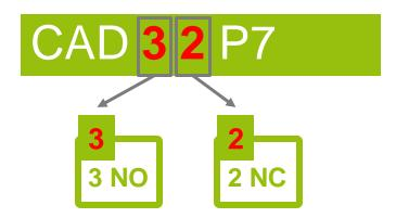
TeSys D auxiliary contactor with 3 NO and 2 NC contacts, 230 V AC coil
