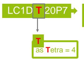
**4P** contactor, 20 A **AC1**, 230 V AC control circuit
