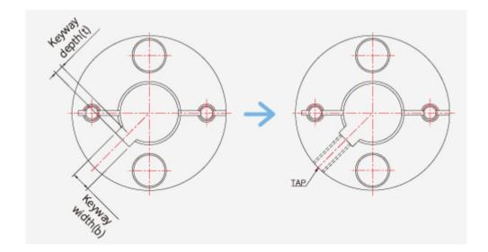
Sung-il Machinery provides additional tapped holes on coupling hubs upon the request.
