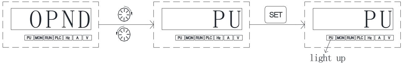
Note: 1.In “PU mode”,parameter unit screen displays **PU**, and the indicating lamp **PU** will light up.
